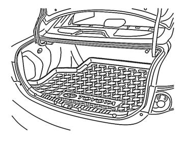
Place cargo tray in trunk area with the logo at the rear of the vehicle as shown. Ensure tray makes full contact with the trunk floor.
